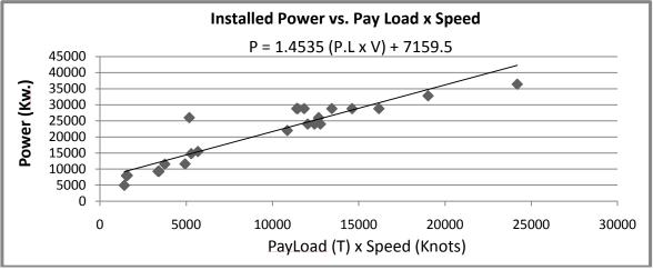
Figure (7): The relationship between Power VS. Payload x Speed
