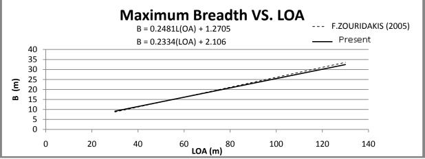
Figure (12): Comparison between ships's B VS. LOA
