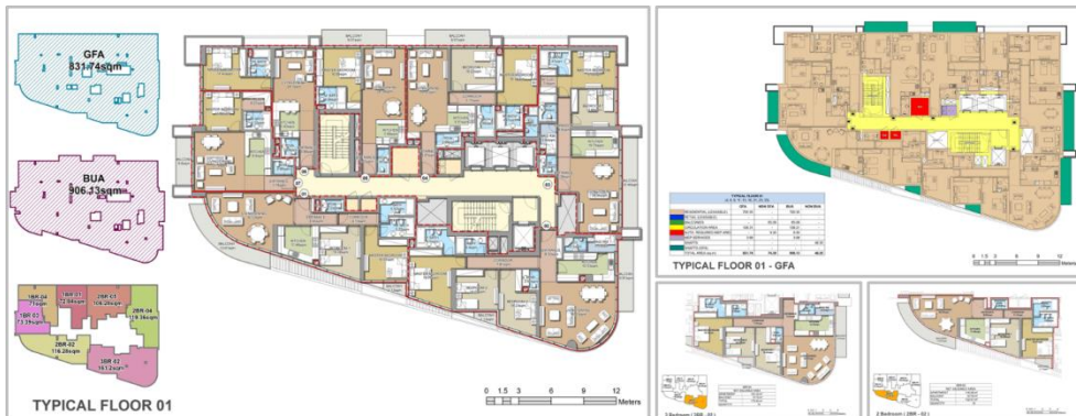
Fig. 14. The automated generated plans showing different types of illustrations and details
