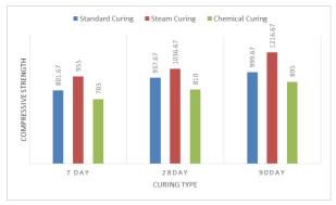
Figure 2: Compressive strength results for mix MO15 underdifferent type of curing
