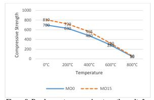
Figure 8: Development compressive strength results for metakaolin concrete under different degrees of temperatures and ordinary Portland cement mixes at
