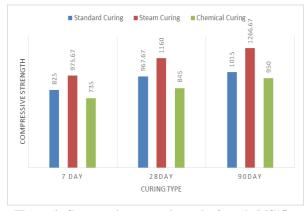
Figure 4: Compressive strength results for mix MS15 under different type of curing
