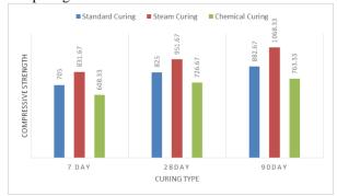
Figure 1: Compressive strength results for mix MO0 under different type of curing
