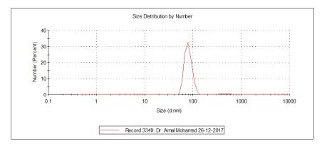
Fig. (1b): Zetasizer average diameter of chitosan NPs.
