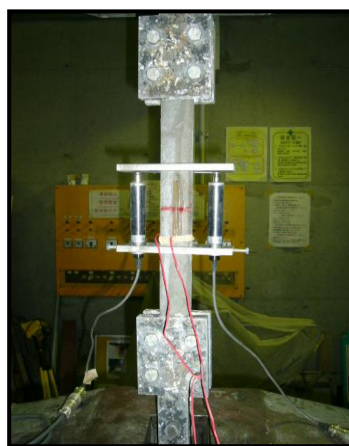
Photo 2: Setup of ferrocement thin plate specimen under direct tension
