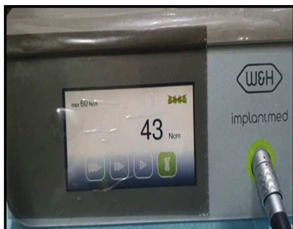
Figure 5: Photograph of the screen of W&H Surgical motor showing the insertion torque measurement from initial insertion to full insertion with peak insertion torque.
