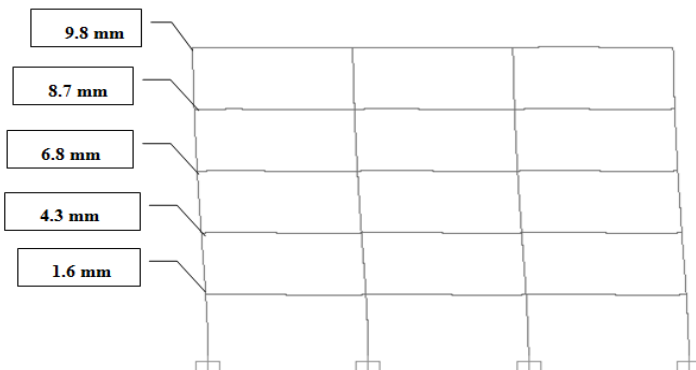
Fig. 27. Top lateral displacement of Frame #3
