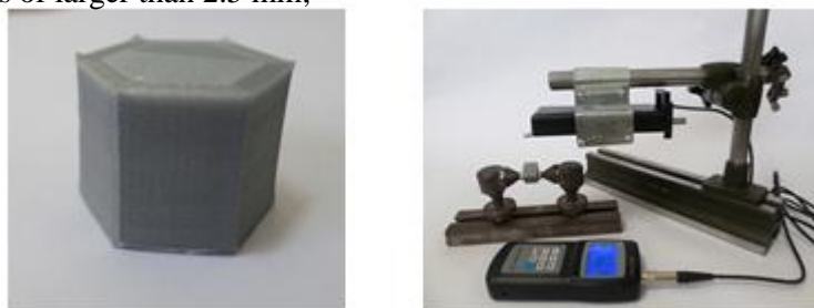
Fig. 4. (a) The test specimen (b) the roughness measuring set up
