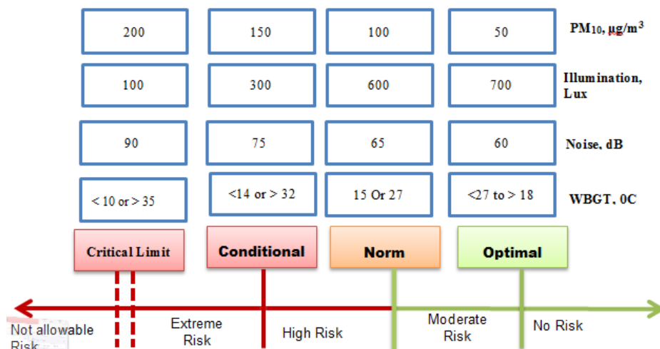
Fig. 3. Modified risk assessment model applied for IAQ factors in addition to noise levels and intensity of light in administration areas [24, 27]
