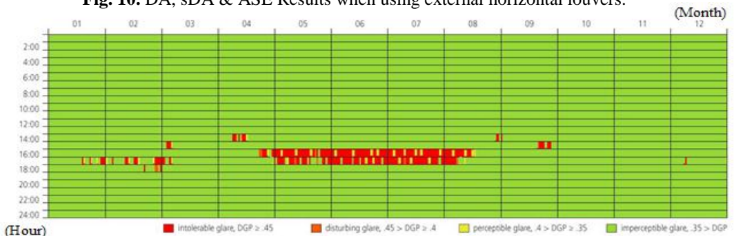
Fig. 11. Annual DGP after adding the external horizontal louvers showing the reduction of glare during May and August.
