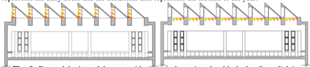
Fig. 9. External horizontal louvers with a vertical spacing that block the direct lighting at 45degrees and 50cm wide (above left) versus internal vertical louvers with a horizontal spacing that block the direct lighting at 45degrees and 50cm deep (above right).
