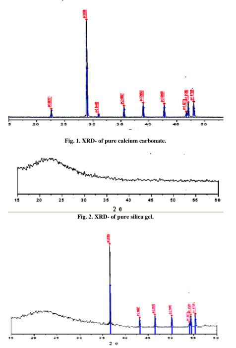
Fig. 3. XRD- of composite of silica gel with calcium carbonate .
