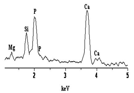
Fig. 9. EDX-spectrum of SiO<sub>2</sub> nanoparticles after 14 days soaking in SBF.
