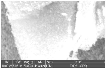
**Fig. 6. SEM-image of silica with calcium carbonate calcined at 550°C.** *Egypt. J. Chem.* **55**, No. 4 (2012)
