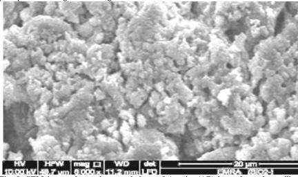
Fig. 8. SEM image shows the morphology of Apatite (AP) layer formed on silica sample after two weeks of soaking in SBF.
