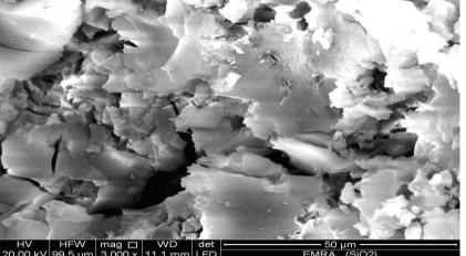
n 3 000 x 11.1 mm LFD EMRA (SiO2) Fig. 5. SEM-image of pure silica calcined at 550°C.
