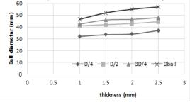
Fig. 15. Flange diameter vs. tube thickness in Flanging (D <sub>ball</sub> = 19 mm, N = 125 rpm and f = 0.125 mm/rev)
