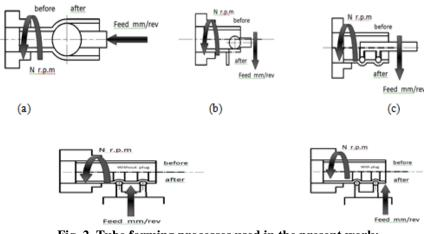
**Fig. 2. Tube forming processes used in the present work:** a) tube end widening, b) tube end flanging, c) in-section widening, e) section throttling and e) joining of an Al tube to a polymer plug
