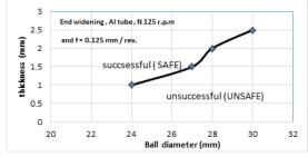
Fig. 10. The limit curve in widening of commercial purity Aluminum
