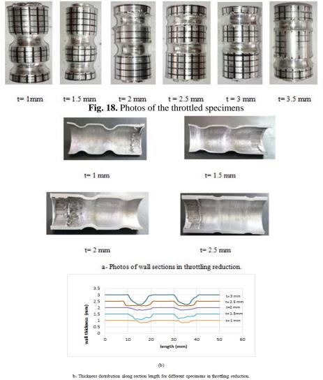
Fig. 19. Photos and plots of thickness distribution along section length for different specimens in throttling reduction.
