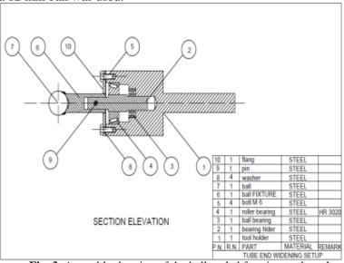
Fig. 3. Assembly drawing of the ball-ended forming tool used
