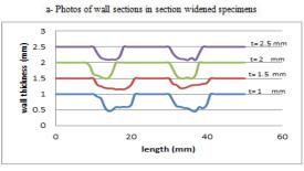
b- Thickness distribution along widened section
