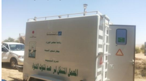
Fig. 2. Mobile lab to monitor air pollution in WAPA
