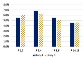
**Fig. 15.** % Difference of story drift of building with openings at third and fourth stories compared with that without opening.
