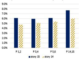
Fig. 17. % Difference of story drift of building with openings at fourteenth and fifteenth stories compared with that without opening.
