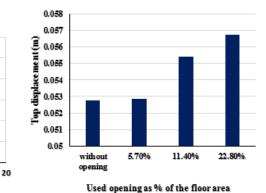
**Fig. 6.** Maximum Displacement for Difference **Fig. 7.** Top Displacement for Difference Area of Openings. Area of Openings.
