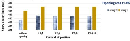
Fig. 18. Story Shear Force for difference Vertical of Position.
