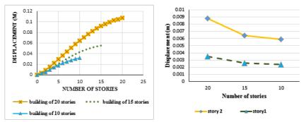
Fig. 21. Story Maximum Displacement in X Direction.
