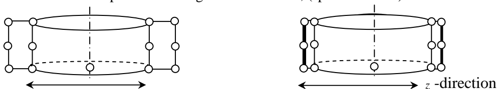
Figure (5-b), Locations of thermocouples on the surface of fins that coincide on x and z axis for the specimen having cylindrical central hole, (specimen no. II).
