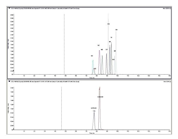
Fig. 2. Typical chromatogram of sulfonamides and trimethoprim.
