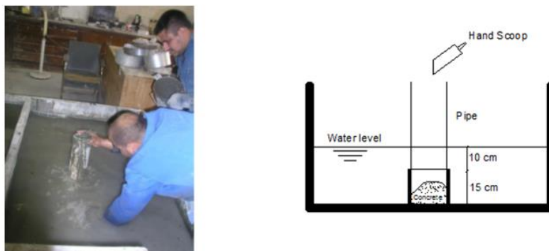
Fig. 1. Underwater casting of concrete samples
