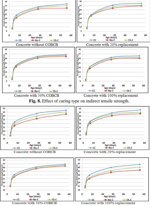
Fig. 9. Effect of curing type on flexural strength.
