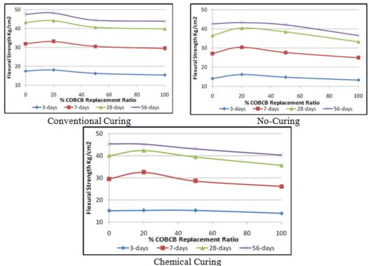
**Fig. 6.** Effect of % (COBCB) on flexural strength.
