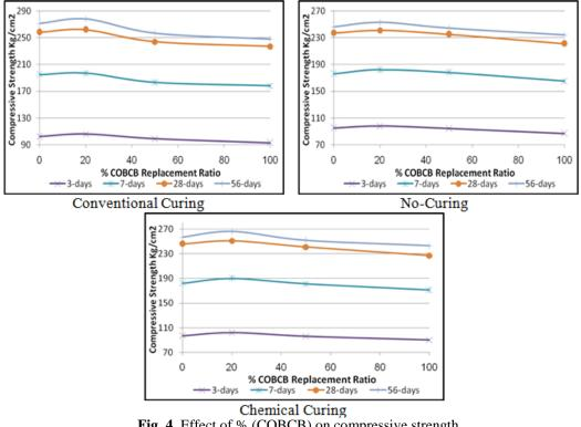
Fig. 4. Effect of % (COBCB) on compressive strength.
