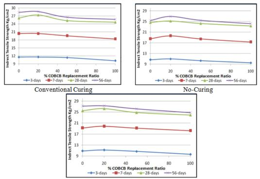
Chemical Curing Fig. 5. Effect of % (COBCB) on indirect tensile strength.
