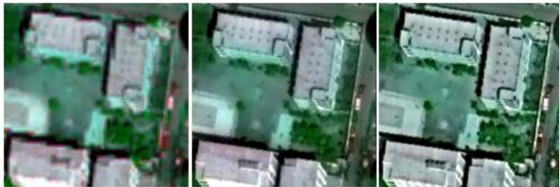
a) BEMD+Wavelet b) BEMD+Curvelet c) proposed BEMD+Shearlet Fig. 4. Comparison of different fusion methods by using WorldView3 images
