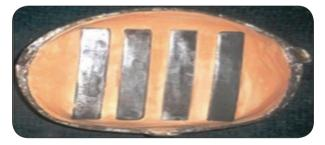
Fig. (1) Stainless-steel patterns invested in dental stone.
