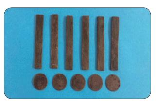
Fig. (4) Finished specimens of PMMA modified by Ag-Nps.
