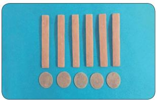
Fig. (2) Finished specimens of conventional PMMA acrylic resin.
