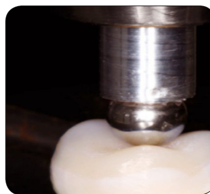
Fig. (2) Load to fracture in the universal testing machine
