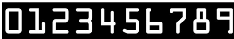
Figure 8: The OCR-A font for the digits 0-9. We will be using this font along with template matching to OCR recharge card digits in images.
