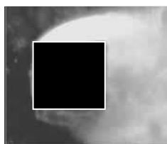
Fig. 7. Cavitation over square-section cylinder, U_o=8.1 m/s, \sigma=2.11 , H=5 mm
