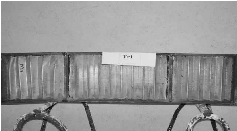
Photo 1: Failure mode of test specimen T_{r1}
