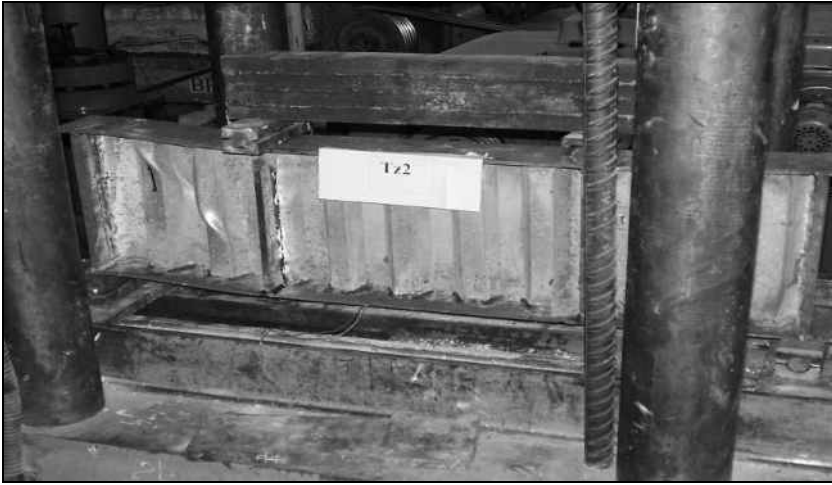
Photo 3: Failure mode of test specimen T_{z2} during test
