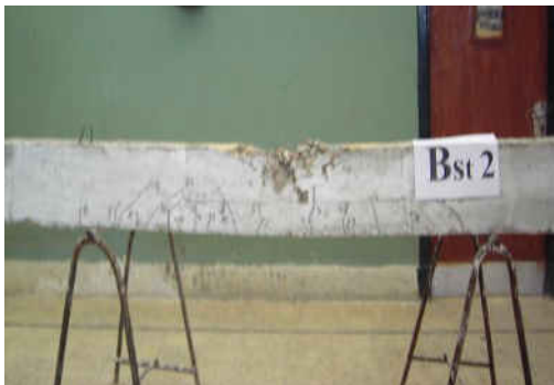
c- Shape of failure of beam (Bst2)
