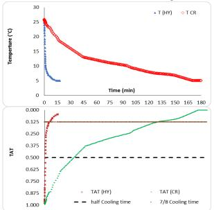
Fig. 1. The combination relationship among cooling time, cucumber temperature and dimensionless of cooling rate
