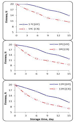
Fig. 6. Effect of storage temperatures on cucumber firmness (N) with HY and CR.
