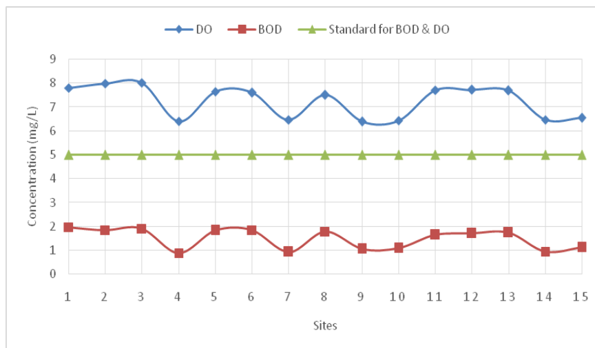
Fig. 2. Variation in average (DO and BOD) in all sites along the river during period study.
