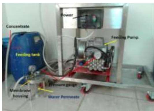
Fig. 2: The laboratory desalination testing unit
