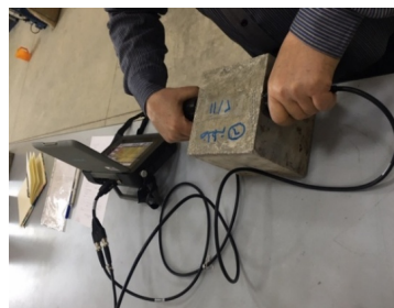
Figure (8), Ultrasonic Pulse Velocity (UPV) test
