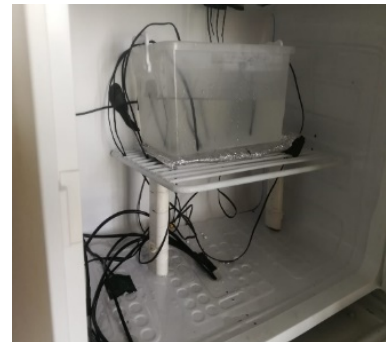
(b) PCM Modified Refrigerator
