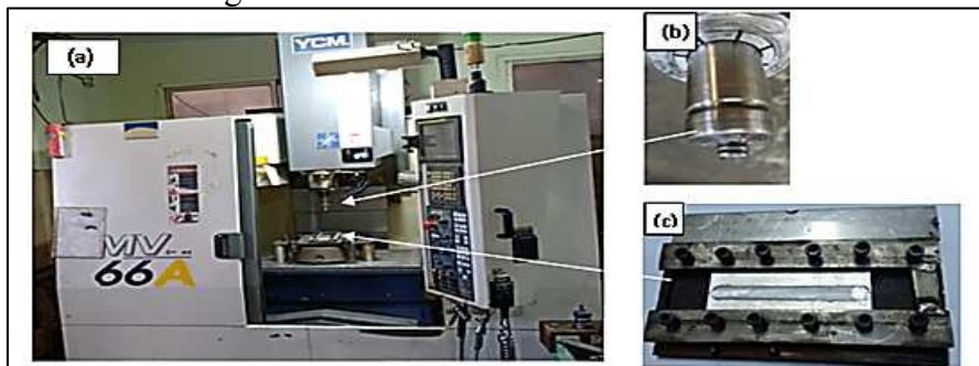
Fig. 4. FSP machine (CNC vertical milling machine) (a), (b) Fabricated FSP tool, and (c) FSP layout. The Fixture was first fixed with help of clamps on the machine bed, and then the plates were properly held in the fixture for FSP. Upon
