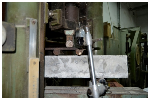
Fig. 5: Flexure test setup
