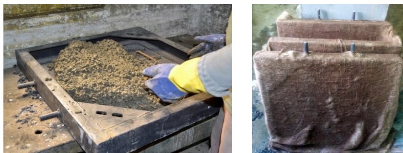
Fig. 4: Typical fabrication process and curing of the (SC) composite cover
