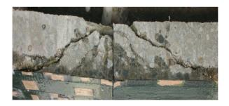
Fig. 13 Punching shear failure
