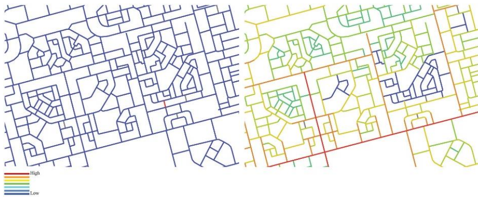
Figure (4) - Space syntax analyses, local integration R500 (left) and global integration Rn (right) in New Damietta city. Source: Authors through depth map software.
