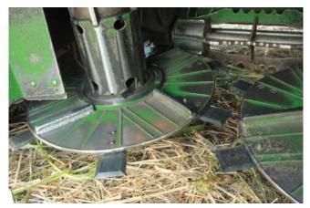
Figure 1 Base cutting unit of a John Deere 3522 sugar cane harvester. (Quick, 1997)
