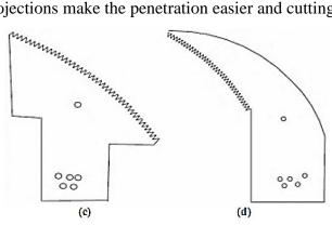
Figure 3 (c) Backward curved serrated-edge blade, (d) forward-curved serrated-edge blade. (Mello and Harris, 2003)
