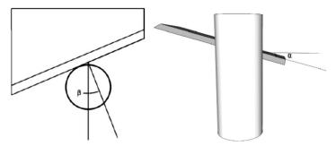
Figure 4 Schematic diagram of a cutting blade design showing the blade oblique angle (β) and tilt angles (α). (Quick, 1997)
