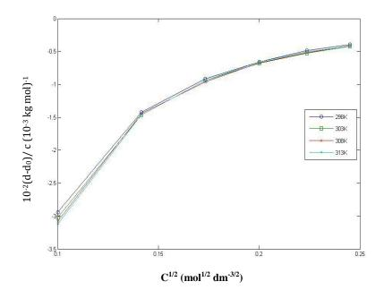
Fig. 2. Plot of  $(d-d_0)/C$  Vs.  $C^{1/2}$  for sodium nitroprusside at different temperatures for 5% weight of methanol.
