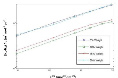
$C^{1/2} \ (mol^{1/2} \ dm^{\cdot 3/2})$  Fig. 5. Plot of (K<sub>s</sub> - K<sup>0</sup><sub>s</sub>)/C Vs. C<sup>1/2</sup> for sodium nitroprusside in various composition of propanol at 303.15K.
