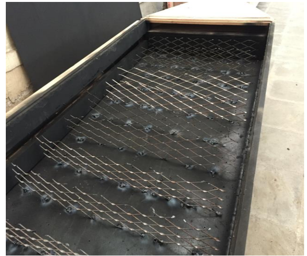
Fig. 4. Photo of wire-mesh position in the collector.
