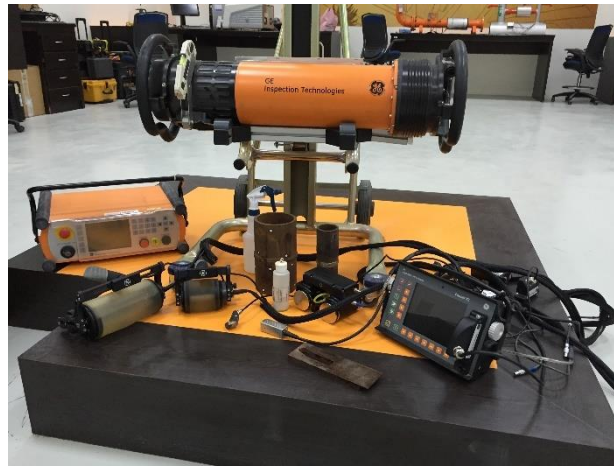
Fig.(1). Photo RT&UT Equipment used.
