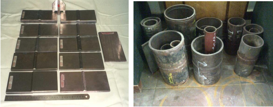
Fig.(2) Photograph of group(A): PETROJET&MASSA butt welded joints with standard & Practical Discontinuities.
