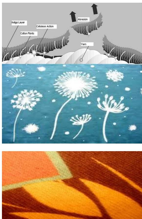
Figure 10: The action of cellulases in discharge printing (a), White discharge printing (b) and Halftone (c)
