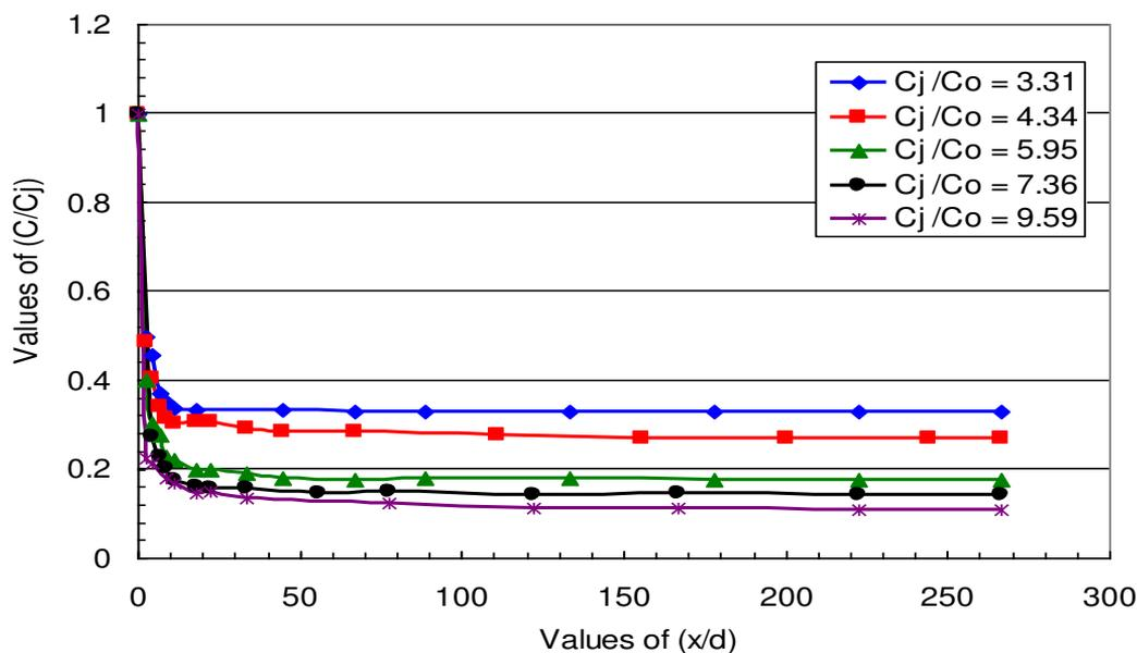
Fig. 8: Relationship between  $C/C_j$  and  $x/d$  for different values of  $C_j/C_o$  at  $\theta=90^\circ$  and  $R=2.73$ .
