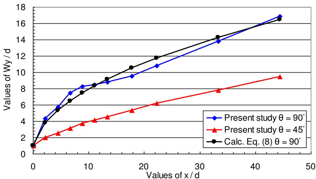
Fig. 9: Influence of jet inclination to the mainstream on growth of jet width for R = 7.30.
