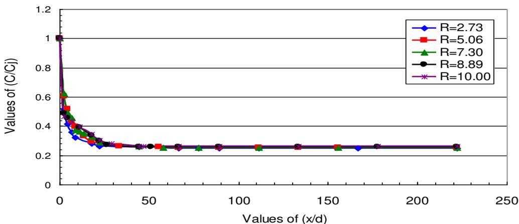
Fig. 7: Relationship between  $C/C_j$  and  $x/d$  for different velocity ratios at  $\theta = 45^\circ$  and  $C_j/C_o = 4.34$ .
