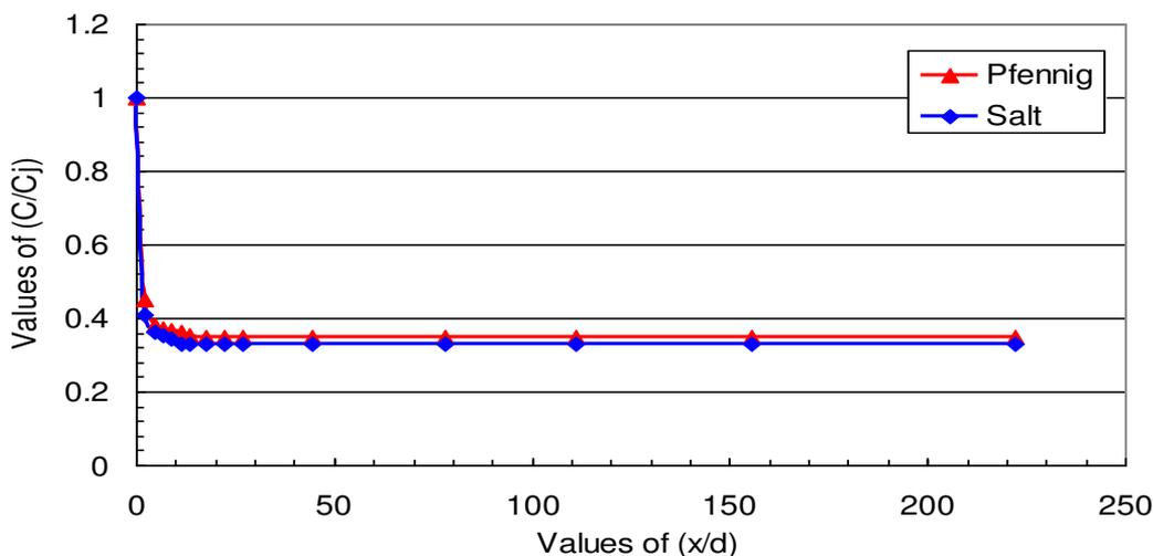
Fig. 6: Relationship between  $C/C_j$  and  $x/d$  for different types of pollutants at  $\theta = 90^\circ$ ,  $C_j/C_o = 2.94$  and  $R = 7.30$ .
