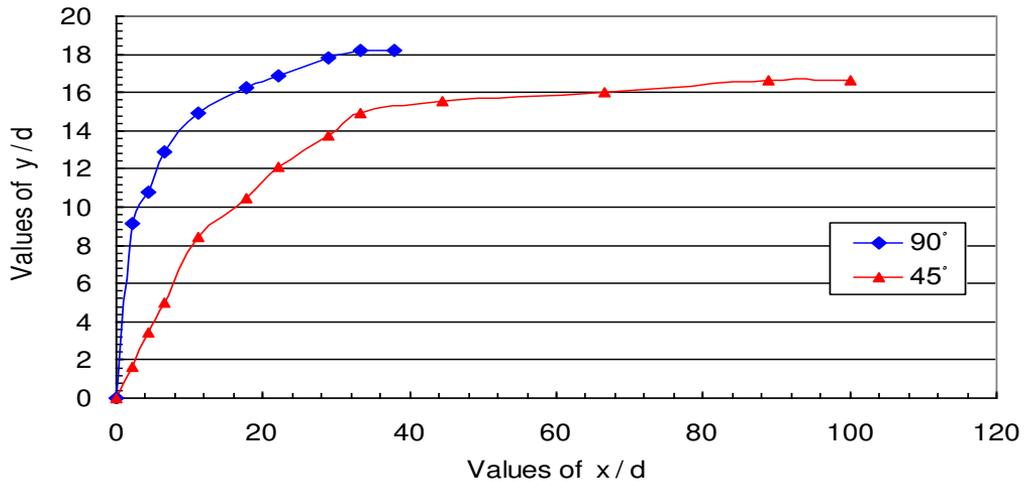
Fig. 3: Influence of jet inclination to the mainstream on jet trajectory for R = 10.00.
