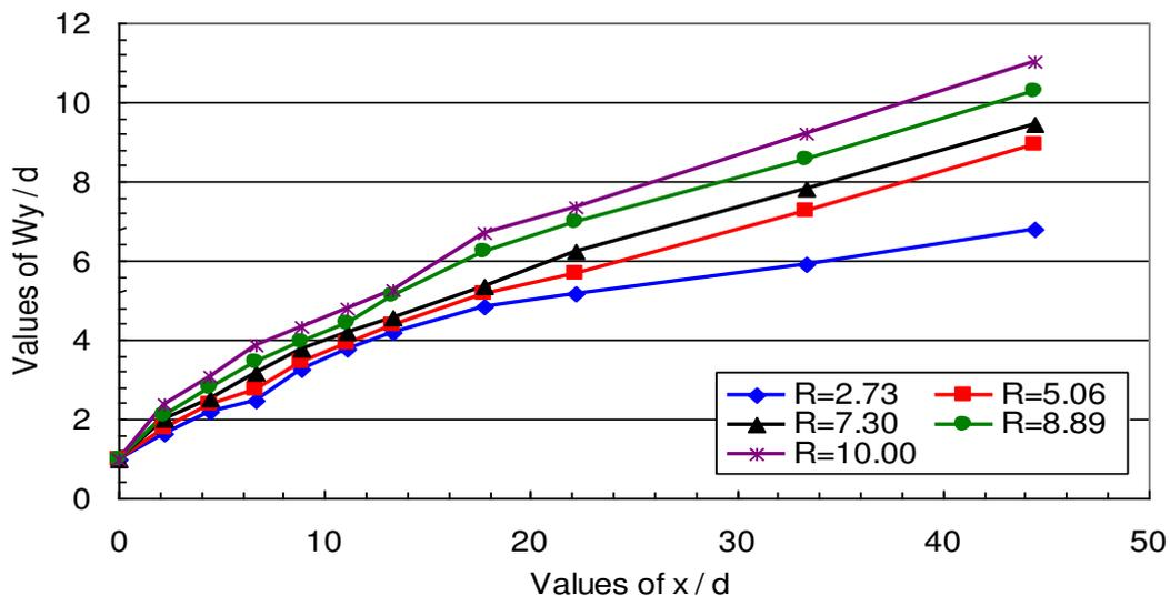
Fig. 10: Relationship between  $W_y/d$  and  $x/d$  for different velocity ratios and  $\theta = 45^\circ$ .
