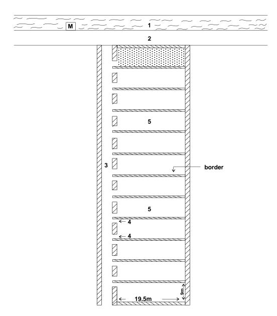
Fig. 2. A sckech map for the study area in a wheat field in the study area, Qalubiya Governorate showing the large irrigation canal, the minor canal and the basins. 1: large irrigation canal, 2: narrow road, 3: minor canal, 4: holes for water entrance, 5: the basins sown with wheat grains, M: irrigation pumping machine.
