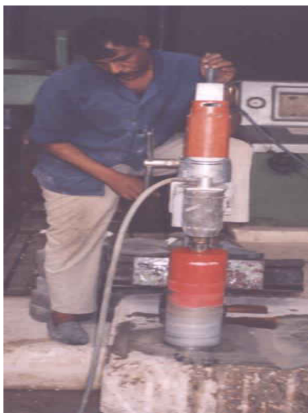
Fig. (1) Drill machine for core samples
