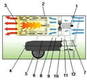
Fig .3. Heat paths in the burner
