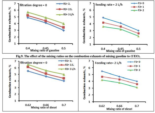
Fig.10. The effect of the mixing ratios on the combustion exhausts of mixing diesel to (UEO).
