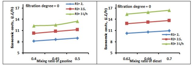
Fig.11. The effect of the mixing ratios on the economic costs of mixing gasoline or diesel to (UEO).
