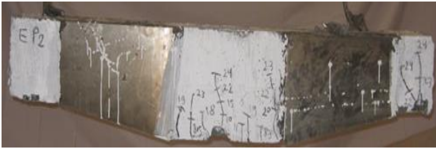
Fig. (48): Crack pattern of beam "EP.2" with thickness of steel plate (1.00 mm)
