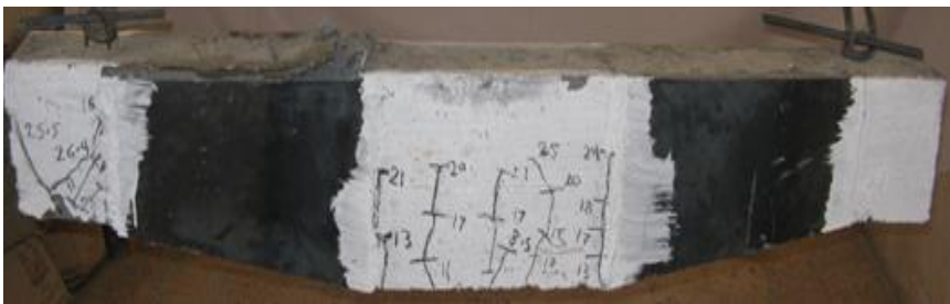
Fig. (47): Crack pattern of beam "EP.1" with thickness of steel plate (1.50 mm)
