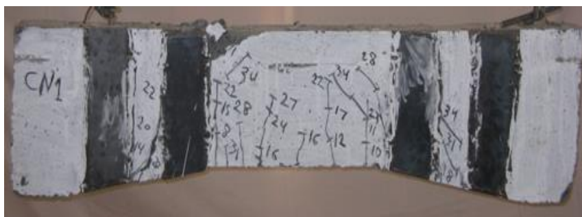
Fig. (3):Crack pattern of beam "CN.1". With thickness of steel plate (2.00 mm)
