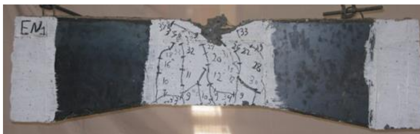
Fig. (15): Crack pattern of beam "EN.1" with thickness of steel plate (1.50 mm)
