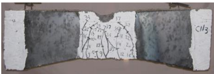
Fig. (5): Crack pattern of beam "CN.3".with thickness of steel plate (2.00 mm)
