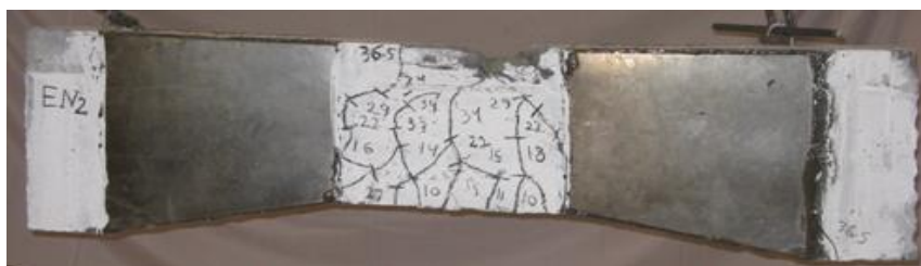
Fig. (16): Crack pattern of beam "EN.2" with thickness of steel plate (1.00 mm)
