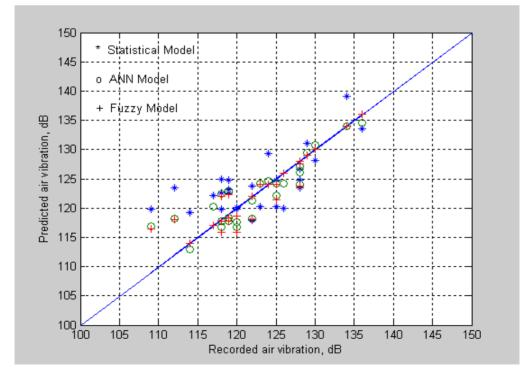
The Fig. 9: Recorded vs. predicted dB for the different models
