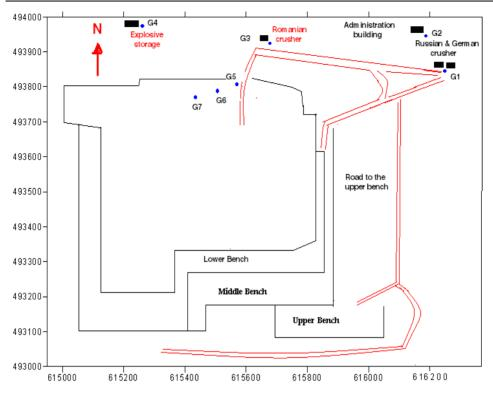
Fig. 1: Layout of the Limestone quarry at ACC
