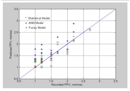
Fig. 8: Recorded vs. predicted PPV for the different models
