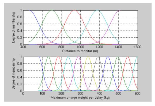
Fig. 4: Membership functions of PPV model inputs
