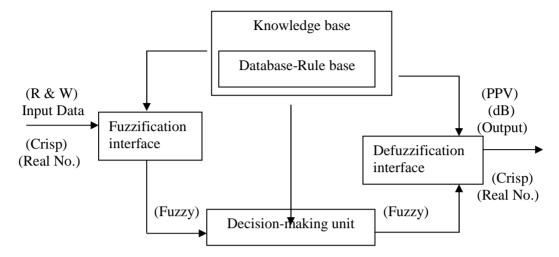
Fig.3: A typical Fuzzy System for Fuzzy Logic Modeling Process.
