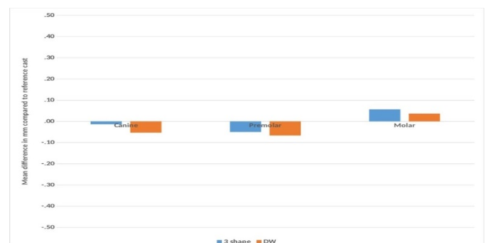
Figure 3: Differences of mesio-distal digital measurements relative to the reference cast (in mm) of the 2 scanners.
