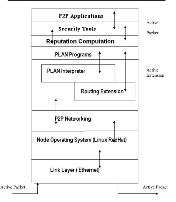
Figure 1: Proposed secure active routing node architecture
