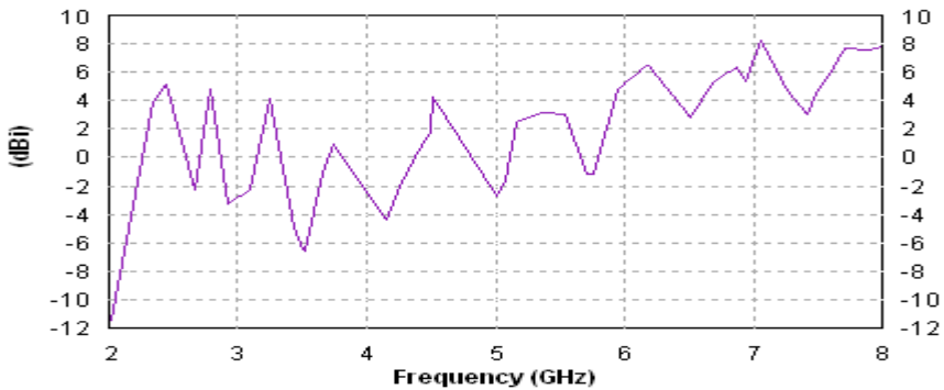
Figure 8. Simulated gain as a function of frequency for the antenna for an arrangement of the slots that construct the shape of the letter C.
