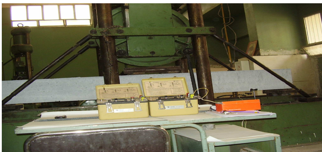
Fig. (2): The beam instrumentation and testing machine.
